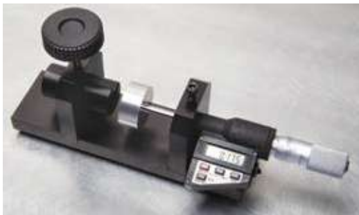
Calibration fixture 2U-16U sensors English/Metric 855578-001
