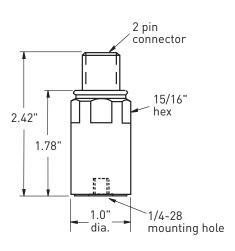
**Notes:** <sup>1</sup> A maximum current of 6 mA is recommended for operating temperatures in excess of 100°C. **Accessories supplied:** SF6 mounting stud; calibration data
