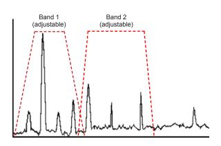
The transmitter has two independent processing bands with flexible mapping options to two separate 4-20 mA analog outputs. The processing channels contain selectable integration, allowing input from accelerometers to be output as acceleration or velocity. Selectable band filters and detector types make it easy to tailor the processing to specific machines or applications.
