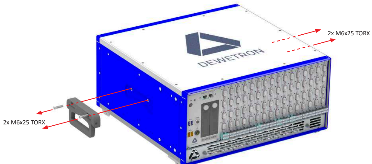
Fig. 9: Demounting the handles
