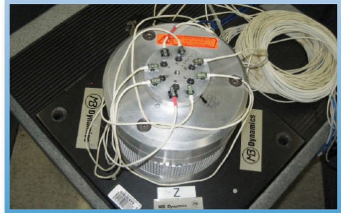
Win475 MDCC mounted with eight (8) piezoresistive accelerometers
