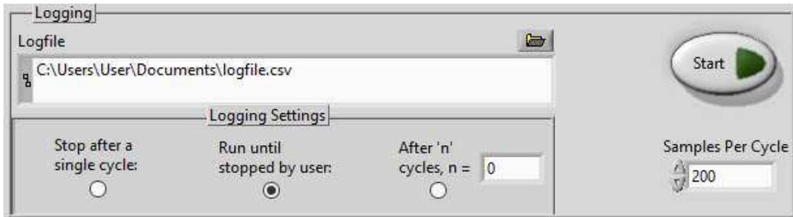
If this window is configured as above, when the start button is pressed, the software will write 200 samples at a time to the file and will keep running until the same button is pressed. For more information, look at the Logging tab section of this manual (section 3.3.3).
