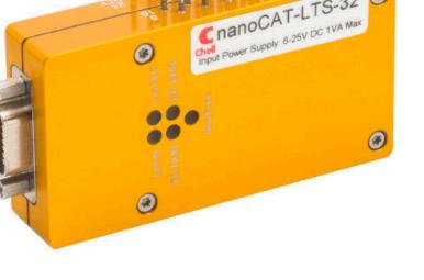
The nanoCAT-LTS-32 makes use of 33 absolute transducers which are thermally compensated and conditioned to provide 32 either absolute or differential measurements relative to the reference port.
