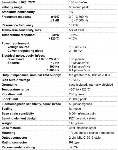
**Notes:** <sup>1</sup> Both calculations are in units of Ohms, f is signal frequency in Hz **Accessories supplied:** #12105-01 captive socket head (metric mounting available); calibration data (level 3)
