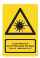
DO NOT STARE INTO BEAM Class 2 Laser Product Laser CLASS 1: invisible,  $\lambda$  = 1550 nm, output power: < 10 mW Laser CLASS 2: visible, green laser,  $\lambda$  = 510-530 nm, output power: < 1 mW
